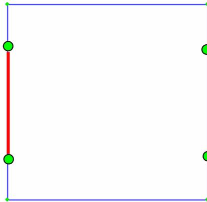
Now position the cursor over the line segment shown above in red, press and hold the left mouse button and drag the section of boundary inward, releasing it when you are happy with the dragged geometry. Repeat the operation on the right hand side.
