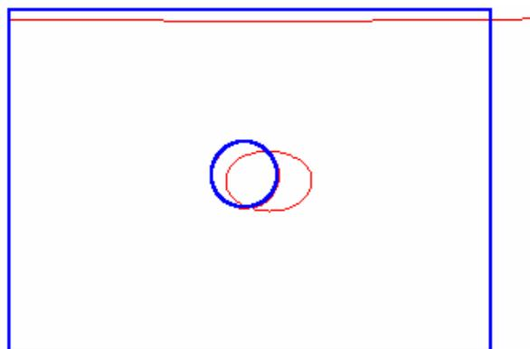
Notice the ovaling of the hole and the fact that the right edge of the plate deforms most in the centre, indicating the reduction in stiffness resulting from the hole.
