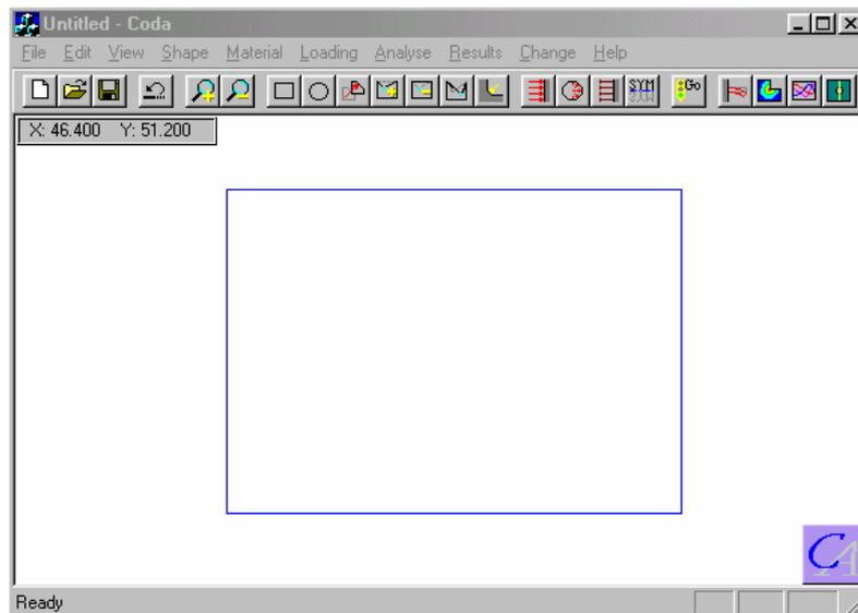
Notice now how the bottom left hand corner of your rectangle is at the origin, i.e. its coordinates are (0,0). The origin automatically snaps to this corner of a rectangle when it is the first shape to be defined.
