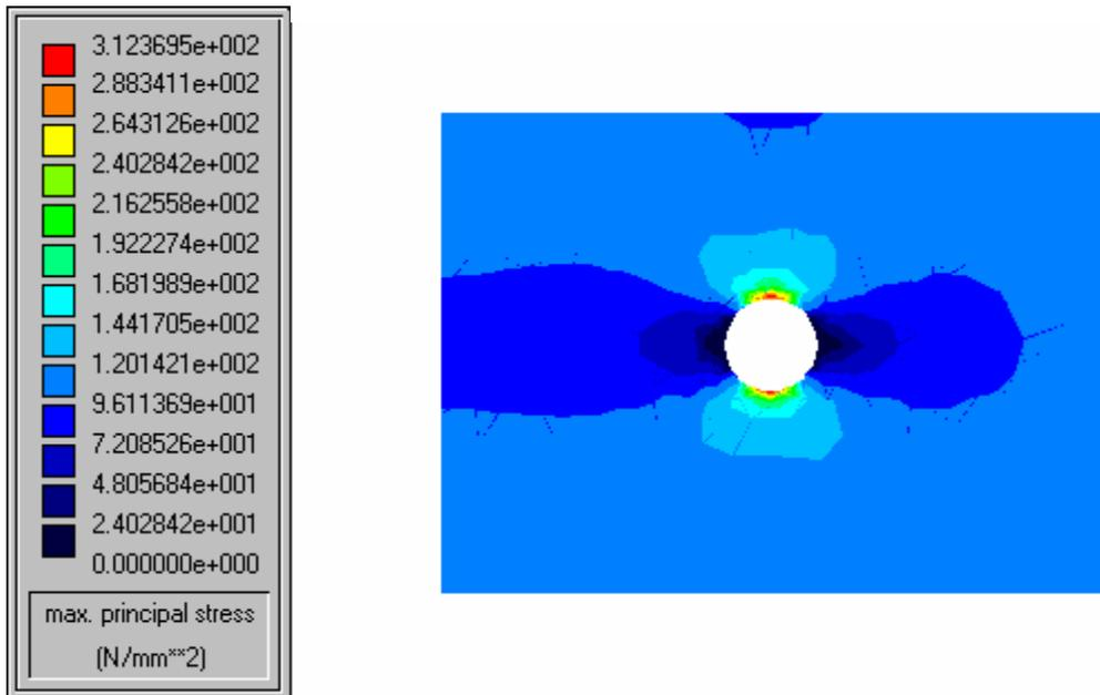
In this example the maximum stress is  $312.4 \text{ N/mm}^2$ , giving a stress concentration factor of 3.124 for the hole. Yours will be somewhat different because you have a different geometry, but the maximum value should be slightly over 300, depending on the size of the circular hole relative to the plate dimensions.
