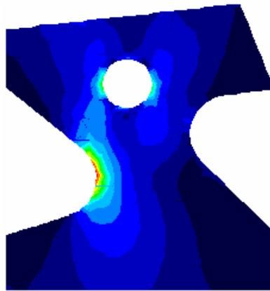
In this example (again, your contour plot will be different, of course), the maximum stress should increase slightly with the addition of the hole, and the hole is clearly attracting stress concentration effects. Zoom in around the stress concentrations to see more clearly the stress distribution.
