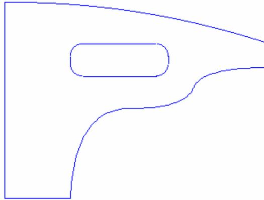
Define a pressure of 600 in the x-direction on the short edge at the right hand side of the bracket, and a pressure of 100 in the y-direction on the top of the hole. We will complete the model with displacement constraints, but this time apply them as symmetry/rollers conditions. This boundary condition constrains an edge against displacement in the direction perpendicular to the line, and this can model either a plane of symmetry or a 'rollers' constraint.
