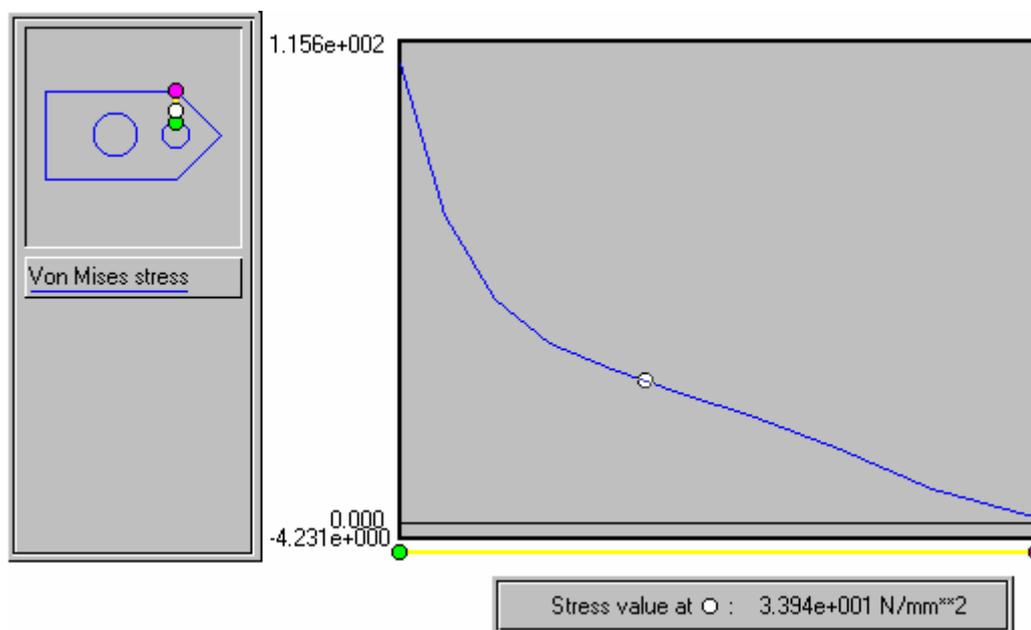
This display works in the same manner as the boundary graph plot seen earlier. The cursor location on the screen is reflected in the white circle on the small model display, to indicate the model location corresponding to the horizontal position in the graph, and the 'Stress value' box indicates the stress level corresponding to the vertical position of the cursor on the graph.
