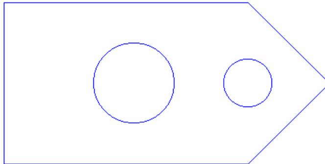
Now we define the loading on the component, which is to take the form of a bearing load through the right hand hole, this representing a normal load in a Cosine distribution over  $180^\circ$  of arc.
