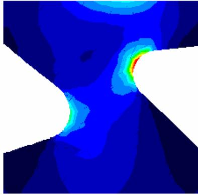
The maximum von Mises stress will have reduced with the increased fillet radius, and indeed the location of the maximum may well have moved to the other fillet. If your maximum stress is still on the same fillet, simply click-and-drag the radius again to a larger radius until the maximum moves to the opposite fillet.
